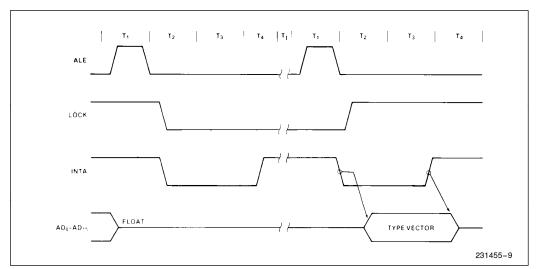
Figure 6. Interrupt Acknowledge Sequence
