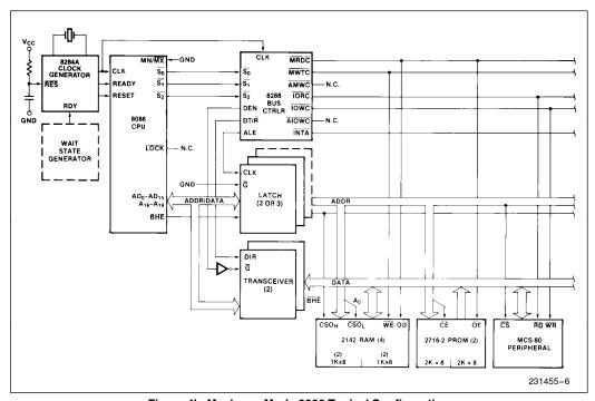
Figure 4b. Maximum Mode 8086 Typical Configuration
