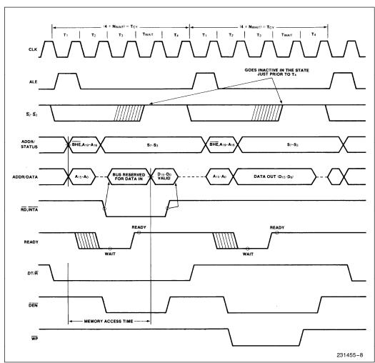
Figure 5. Basic System Timing
