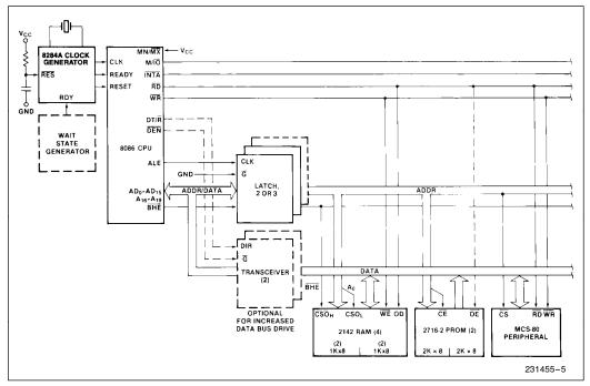
Figure 4a. Minimum Mode 8086 Typical Configuration
