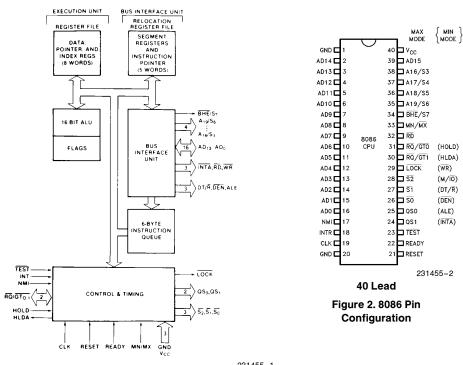
Figure 1. 8086 CPU Block Diagram
